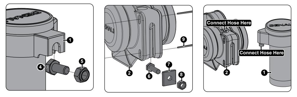
**Compressor Mounting:** Use the M8 bolt (#4) and nut (#5) to secure the compressor to you motorcycle. The compressor should be mounted so that the cylinder is vertical with no more than a 25 degree variance from the vertical position.
